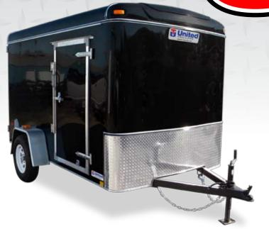
The ULH by United Trailers is perfect for the person who wants a quality-built trailer at an unbeatable value. The ULH is loaded with impressive features such as .030 aluminum exterior, 3/8 "plywood interior walls, TSR vents and 12 volt dome light with switch. When you want exceptional value, look no further than the ULH.
